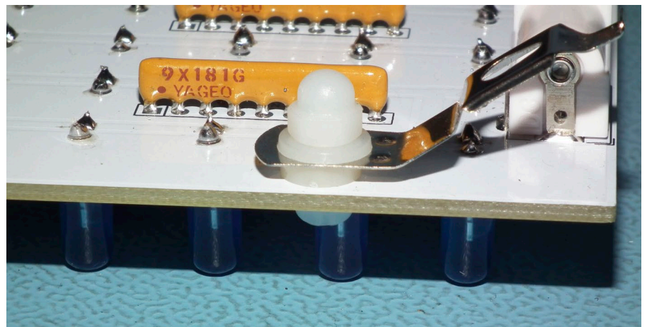
Closeup showing the detail on how to fit the clips from the Rinkit frame to the PCB.
